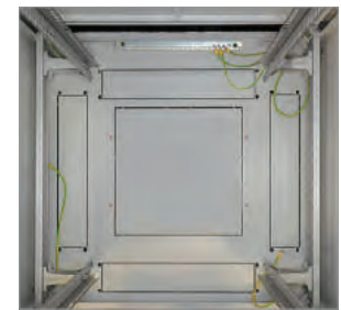
Cabinet bottom with pre-assembled earthing bar, surrounding cable entries and pre-punched opening A (380 x 380 mm)
