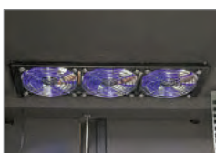
Rear-sided roof area with 3 x super-silent fan
