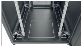
Cabinet bottom with pre-assembled earthing bar, surrounding cable entries and pre-punched opening A (380 x 380 mm)
