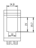
Type of DIN-rail adapter Article no. Type of fastening Material Title max. Keystone Stainless Steel DIN-Rail DIN-Rail 35 mm 1 AD25184 straight metal Adapter for 1 x Keystone Stainless Steel DIN-Rail 2 ET-25184.1V2 DIN-Rail 35 mm straight metal Adapter for 2 x Keystone 3 ET-25184.2V2 Stainless Steel DIN-Rail DIN-Rail 35 mm straight metal Adapter for 3 x Keystone
