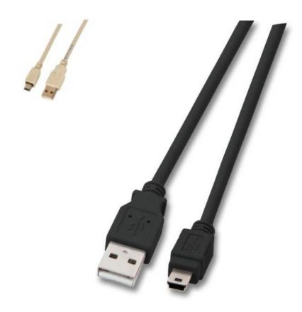
Supports data transmission rates up to 480 Mbit/s. Wire diameter: AWG28 / AWG24. Shielded: folie + braiding. Plug moulded.
