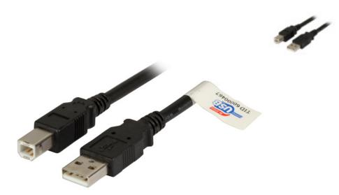
For data transmission rates up to 480 Mbit/s. Wire construction: AWG28 / AWG20. Shielded: Foil + 80% braiding. Plug moulded.
