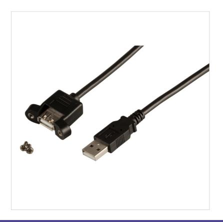
Supports data transmission rates up to 480 Mbit/s. Wire construction: AWG28 / AWG24. Shielded: folie + braiding. Plug moulded.
