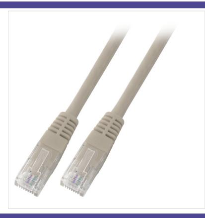
1 Gigabit Ethernet patch cable, unshielded 2 x RJ45 plug, IEC 60603-7 U/UTP 4 x 2 x AWG24/7 PVC Ø=5.4 mm Flame retardant IEC 60332-1 TIA/EIA 568B coded Assembling strain relief with latch protection
