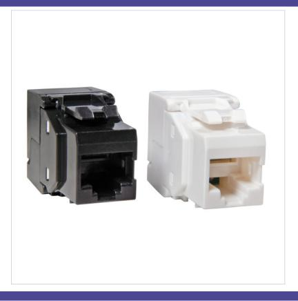
Cat.6 DELTA certified (de-embedded) according to ISO/IEC11801 2nd Edition 2002. RJ45 keystone UTP for AWG24/1 .. AWG22/1. Tool-less assembling. Pair management toLSA-terminal, 568A/B coded. Strain relief via cable tie. PoE Plus according to IEEE 802.3at.
