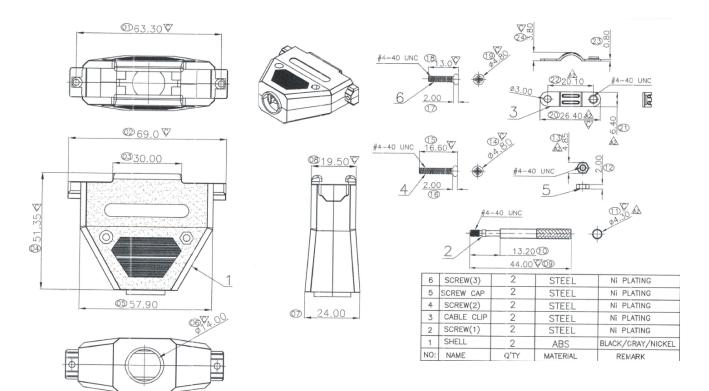
NOTES: 1.ALL DIMENSION MARKED  $\nabla$  MUST BE CONTROLED BY QIP. 2.ALL DIMENSION MARKED  $\otimes$  SHOULD BE MEASURED BY FAI.
