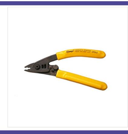
Class stripping tool with 140 $\mu$  opening for stripping the primary coating 250 $\mu$  to 125 $\mu$ Second opening for stripping the 2-3 mm outer jacket With cutting device:FalseWith strip function:True
