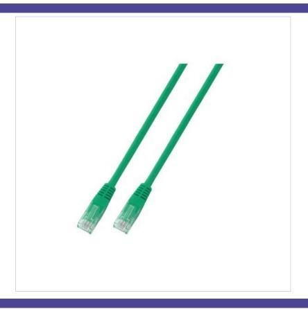
1 Gigabit Ethernet patch cable, unshielded 2 x RJ45 plug, IEC 60603-7 U/UTP 4 x 2 x AWG24/7 PVC  $\varnothing$ =5.4 mm Flame retardant IEC 60332-1 TIA/EIA 568B coded Moulded strain relief without latch protection
