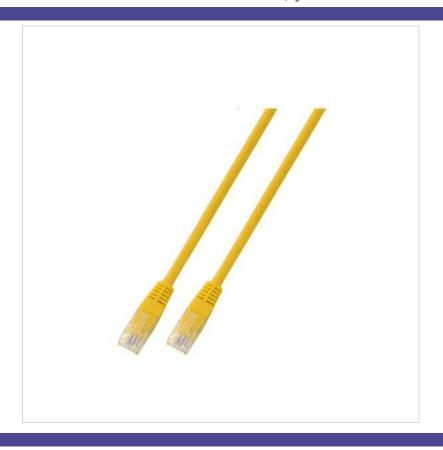
1 Gigabit Ethernet patch cable, unshielded 2 x RJ45 plug, IEC 60603-7 U/UTP 4 x 2 x AWG24/7 PVC  $\emptyset$ =5.4 mm Flame retardant IEC 60332-1 TIA/EIA 568B coded Moulded strain relief without latch protection
