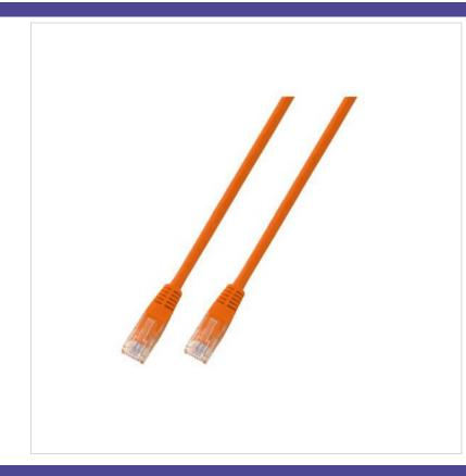
1 Gigabit Ethernet patch cable, unshielded 2 x RJ45 plug, IEC 60603-7 U/UTP 4 x 2 x AWG24/7 PVC Ø=5.4 mm Flame retardant IEC 60332-1 TIA/EIA 568B coded Moulded strain relief without latch protection
