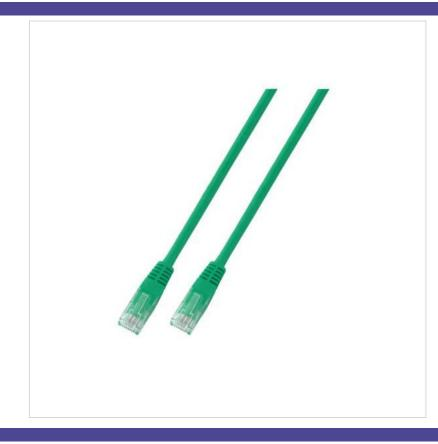
1 Gigabit Ethernet Cat.6 250 MHz patch cable, unshielded 2 x RJ45 plug UTP, IEC 60603-7 U/UTP 4 x 2 x AWG24/7 PVC Ø=5.9 mm Flame retardant IEC 60332-1 TIA/EIA 568B coded Moulded strain relief without latch protection
