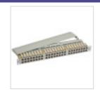
High-Shielded Class E 250MHz patchpanel according to ISO/IEC 11801 and EN50173 for the use in structured cabling systems. Wire connection over LSAterminal AWG22-AWG24. With sheath clamp for earthing. Strain relief via cable tie.
