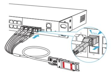
Removing a Duplex LC Cable of 1-8 Breakout AOC.
