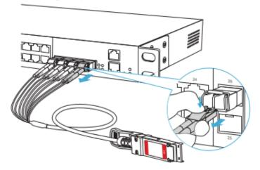
NOTE: Please remove the dust cap before installation and the connector clip should be upward when inserting.
