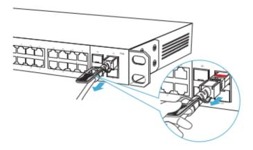
NOTE: When inserting into the upper port, the label should face up. Instead the label should face down when inserting into the lower port.
