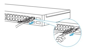
NOTE: When inserting the 40G/100G DAC or AOC, the label should face down.
