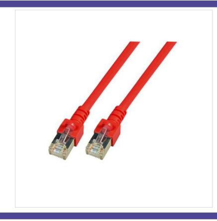
1 Gigabit Ethernet Cat.5e 100 MHz patch cable. 2 x RJ45 plug shielded, IEC 60603-7-3, SF/UTP 4 x 2 x AWG26/7 PVC Ø=5.7 mm, foil and braid shielded. TIA/EIA 568B coded, flame retardant IEC 60332-1. Moulded strain relief boot with latch protection.
