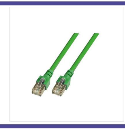
1 Gigabit Ethernet Cat.5e 100 MHz patch cable. 2 x RJ45 plug shielded, IEC 60603-7-3, SF/UTP 4 x 2 x AWG26/7 PVC Ø=5.7 mm, foil and braid shielded. TIA/EIA 568B coded, flame retardant IEC 60332-1. Moulded strain relief boot with latch protection.
