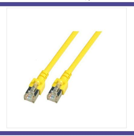
1 Gigabit Ethernet Cat.5e 100 MHz patch cable 2 x RJ45 plug shielded, IEC 60603-7-3 F/UTP 4 x 2 x AWG26/7 PVC  $\emptyset$ =5.6 mm, foil shielded TIA/EIA 568B coded, flame retardant IEC 60332-1 Moulded strain relief boot with latch protection
