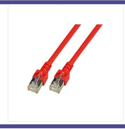
1 Gigabit Ethernet Cat.5e 100 MHz patch cable 2 x RJ45 plug shielded, IEC 60603-7-3 F/UTP 4 x 2 x AWG26/7 PVC Ø=5.6 mm, foil shielded TIA/EIA 568B coded, flame retardant IEC 60332-1 Moulded strain relief boot with latch protection
