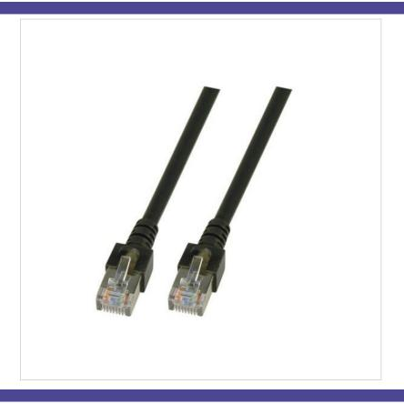
1 Gigabit Ethernet Cat.5e 100 MHz patch cable 2 x RJ45 plug shielded, IEC 60603-7-3 F/UTP 4 x 2 x AWG26/7 PVC  $\varnothing$ =5.6 mm, foil shielded TIA/EIA 568B coded, flame retardant IEC 60332-1 Moulded strain relief boot with latch protection
