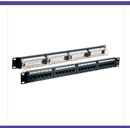
Unshielded Cat.5 100 MHz patchpanel with 24 x unshielded RJ45 jacks. Class D(100 MHz) acc. ISO/IEC 11801 and EN50173. With 8-pole LSA terminals vertical designed, for AWG22-AWG24 wire. 19" steel plate housing. Strain relief via cable tie.
